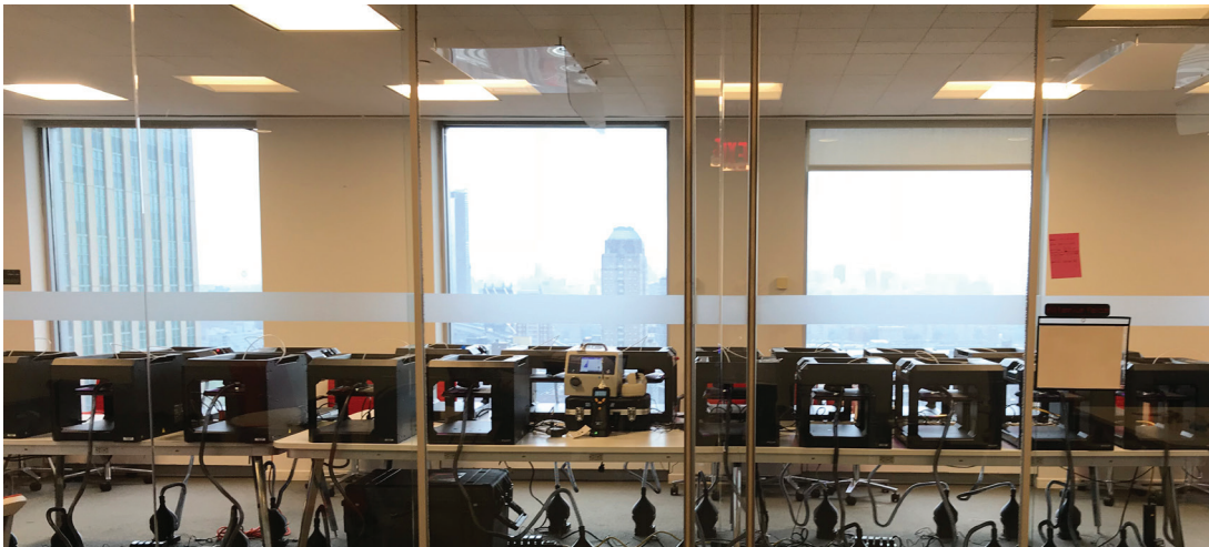
Figure 7. Twenty MakerBot Replicator+ 3D printers equipped with individual local exhaust ventilation (LEV) engineering controls in a conference room [Dunn et al. 2020b].
