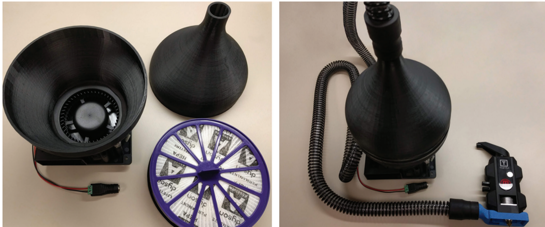
Figure 6. Low-cost air cleaner assembly connected to a modified extruder cover [Dunn et al. 2020b].
