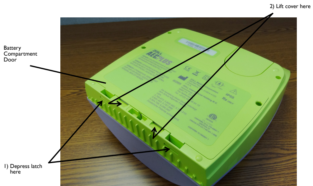
Figure 7: Removing the Battery Compartment Door
